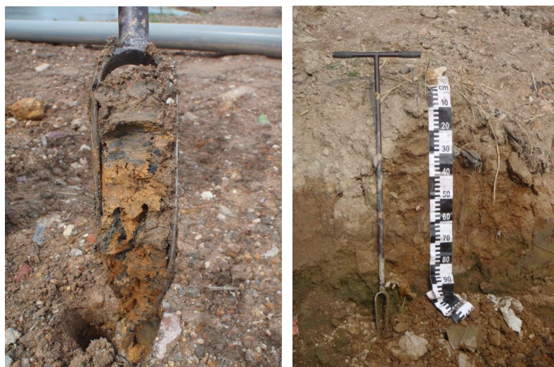
Figure 2. Soil horizons showing layers of filled soils
