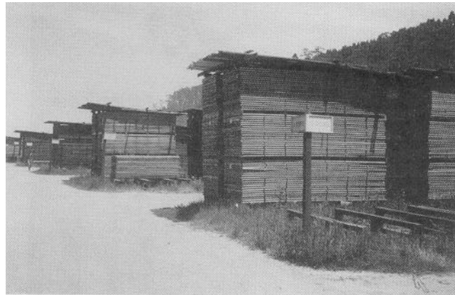
Figure 30-Modern steam kilns in Guatemala (top). Air drying of eucalyptus lumber Lota, Chile; Forestal Rolcura, S.A. Eucalyptus globulus (bottom). (M90 0116, M90 0140)
