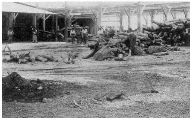
Figure 18-Quebracho in Argentina to be extracted for tannin (early part of century). Photo courtesy of Samuel J. Record collection at U.S. Forest Products Laboratory, Madison, Wisconsin. (M90 0114)
