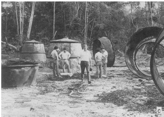
Figure 19-Building of a brick charcoal kiln at La Selva, Veracruz, Mexico (a). Steel charcoal kilns in Venezuela in various stages of operation (b) and assembly (c). Brick charcoal kiln in Venezuela, showing a kiln nearly loaded and ready for bricking shut (d), with door sealed ready for burning (e). Battery of brick charcoal kilns in Venezuela in various stages of operation (f). (M90 0138, M90 0162, M90 0121, M90 0145, M90 0169, M90 0122)
