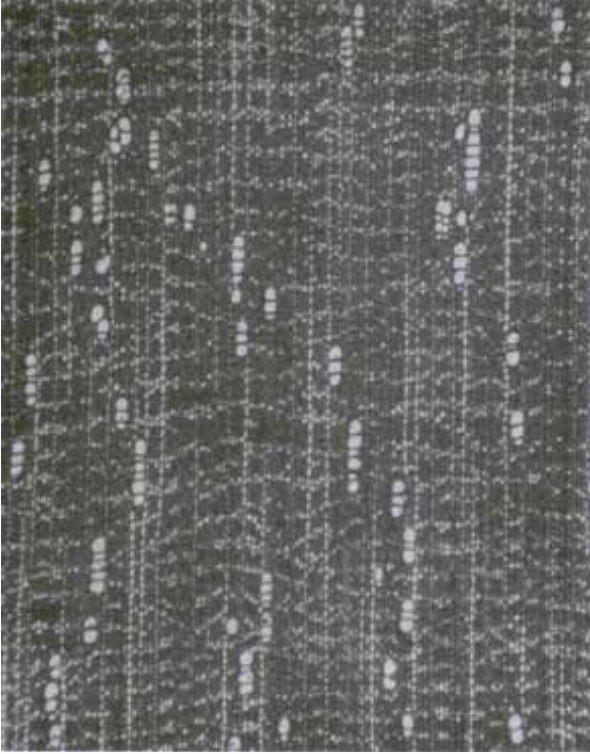
Figure 1.-- Pradosia lactescens , pore and parenchyma arrangement (RBw5975, Bahia) X 30.
