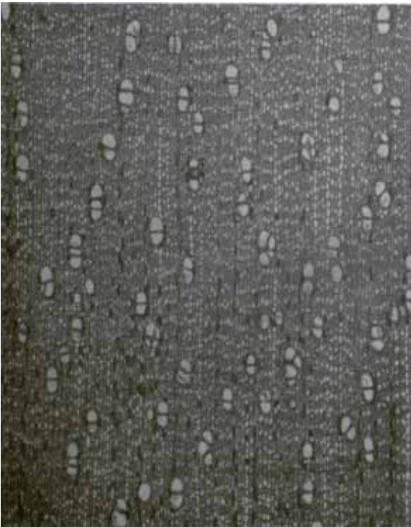
Figure 3.-- P. ptychandra , pore and parenchyma arrangement (BAFOG 55, French Guiana) X 30.
