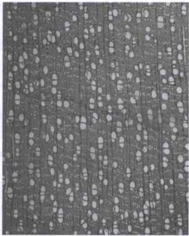
Figure 6.-- P. inophylla , pore and parenchyma arrangement (Ducke 264, Amazonas) X 30.
