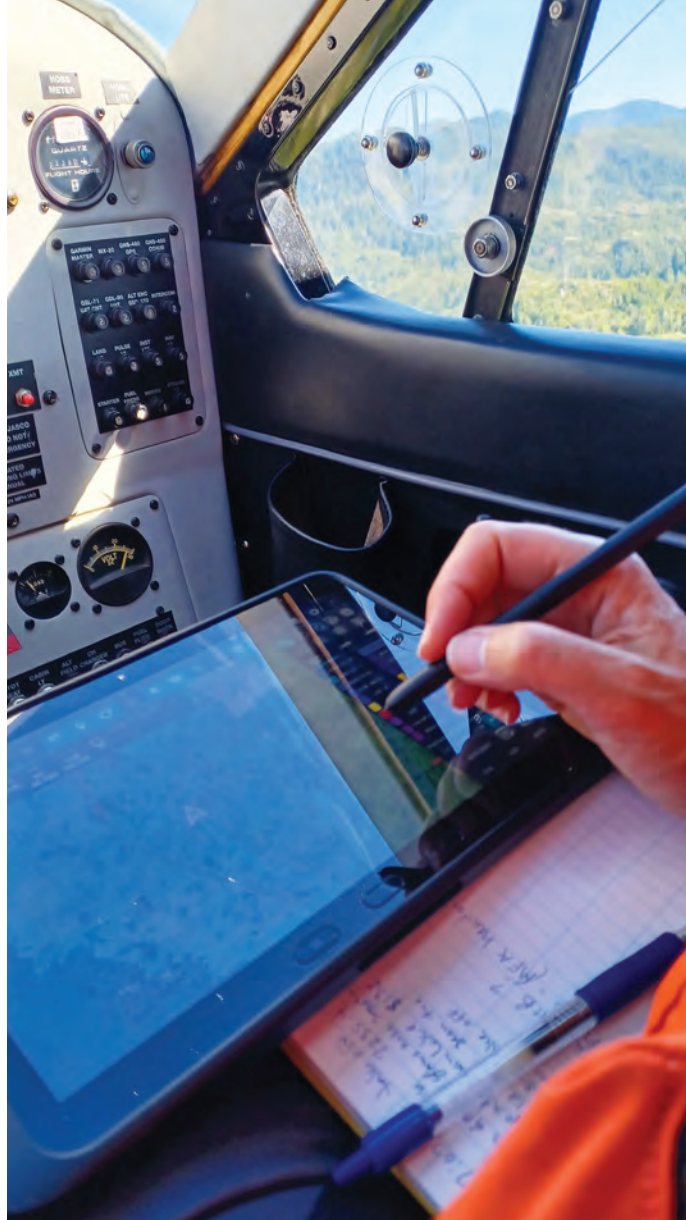
Figure 100. Damage area polygons are drawn on a digital 1:63,000 USGS quadrangle map. Integrated GPS allows surveyors to see the location of the aircraft on an active basemap or satellite image. This feature allows for a more accurate placement of damage area polygons. USDA Forest Service photo by Dr. Karen Hutten.
