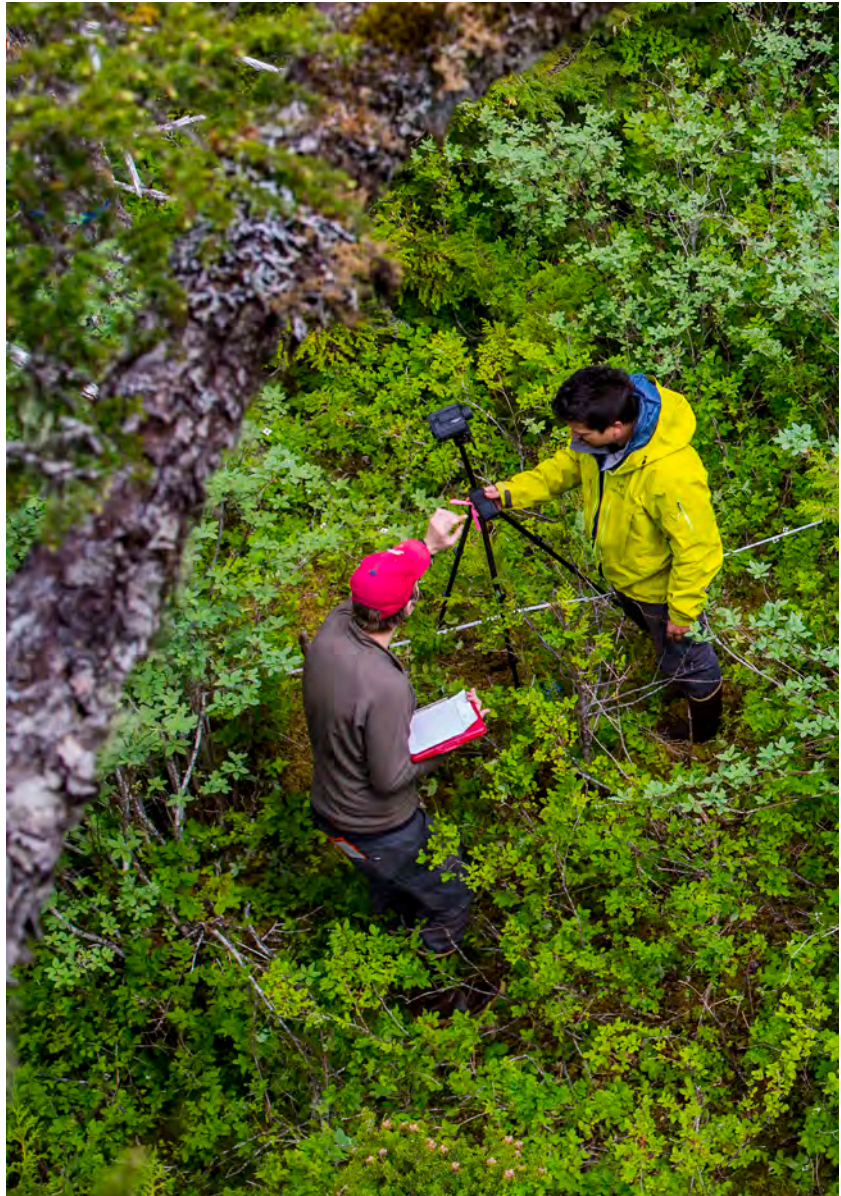
Figure 32. John Krapek and Alex Botelho adjust survey equipment used to stem-map trees, saplings and seedlings in yellow-cedar stands near Juneau. Photo credit: Mark Rainery, University of Alaska Southeast.
