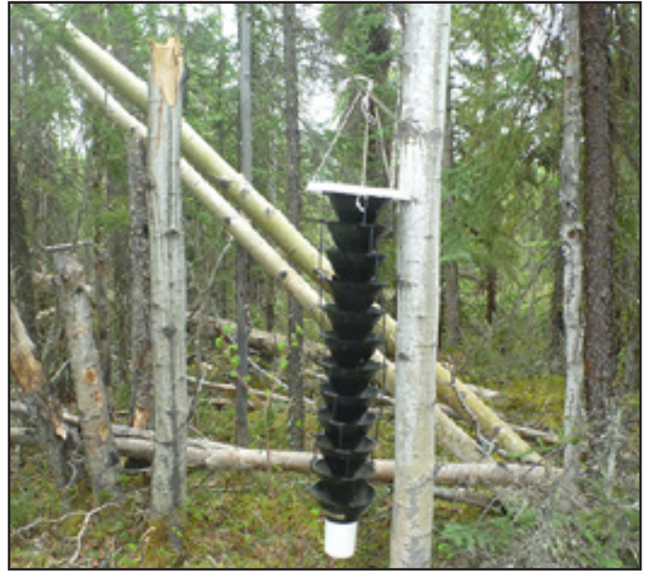
Figure 5: Lindgren funnel traps are commonly used to capture bark beetles. The design is meant to mimic the silhouette of a tree and is baited with attractive compounds.
