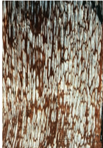
Figure 94. Typical white pocket rot of Porodaedalea (Phellinus) pini with white pockets bordered by reddish, relatively undecayed wood. Photo: Jim Worrall, USDA Forest Service.
