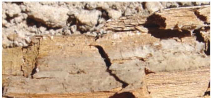
Figure 58. Gray-brown mycelium associated with brown cubical rot. Photo: Jim Worrall, USDA Forest Service.
