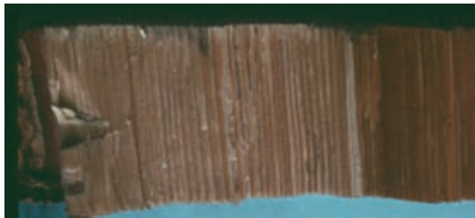
Figure 280. Wetwood in radial section of white fir. Note the narrow, dry transition zone between sapwood on left and wetwood. Photo: Jim Worrall, USDA Forest Service.
