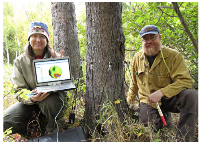
Figure 50. Lori Winton and Steve Swenson use an ArborSonic acoustic tomograph to view internal decay of a live white spruce.
