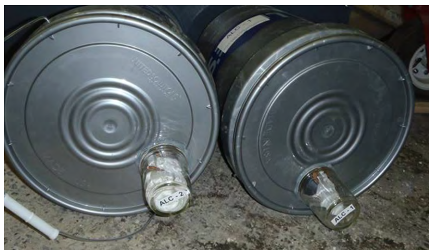
Figure 9. A rearing chamber made from five-gallon plastic buckets, designed to capture wood borers emerging from firewood. Photo by Mia Kirk, AK DNR.
