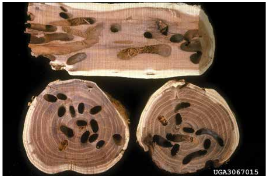
Figure 6. Locust borer larval galleries seen in cross and lateral sections. (James Solomon, USDA Forest Service, Bugwood.org)
