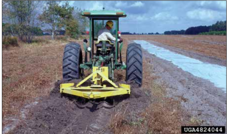
Figure 5. “Scalping” is the use of machinery to remove a thin layer of thatch and top soil before planting a new block of pine seedlings. (Edward L. Barnard, Florida Department of Agriculture and Consumer Services, Bugwood.org)
