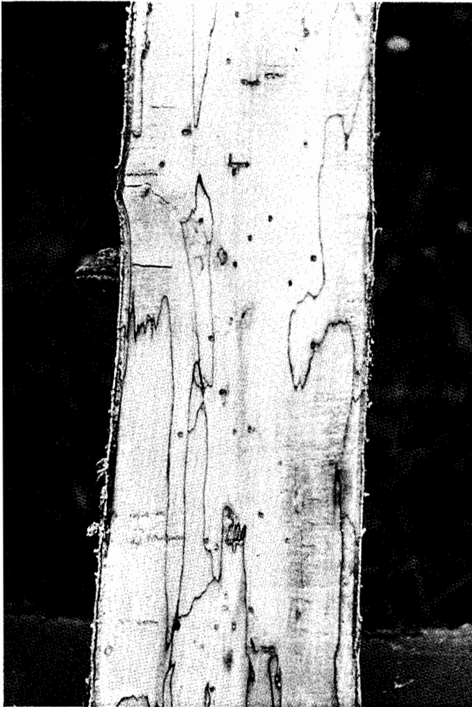
Figure 55.—Initial stage of decay in birch ( Betula pendula ) caused by Fomes fomentarius .
