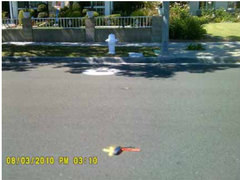
Figure K.7: A good photo of clearly marked point center and includes a permanent object as reference.
