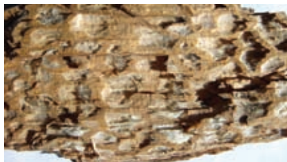
Figure 65. Big white pocket rot. Pockets are up to \frac{3}{8} inch (1 cm) wide and many have white cellulose remains. Photo: Jim Worrall, USDA Forest Service.
