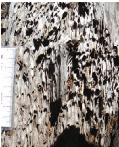
Figure 66. Big white pocket rot. Decayed wood has weathered, leaving relatively sound wood between the pockets. Photo: Jim Worrall, USDA Forest Service.
