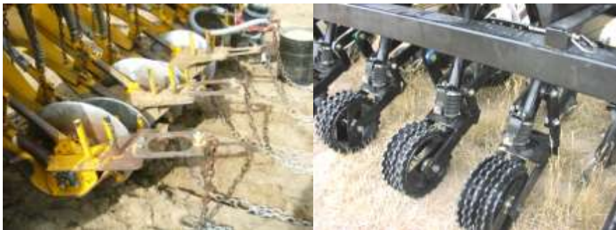
Figure 2. Chains on rangeland drill (left) and imprinter units on minimum-till drill (right)
