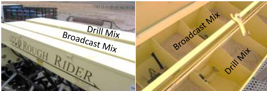
Figure 1. Triple seed box used on both the minimum-till drill (left) and rangeland drill (right).
