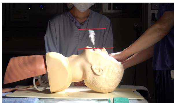
Figure 1. Image of Airflow with test smokes. The airflow in the operating room can be evaluated under various conditions using a test smoke that simulates the patient's exhalation.
