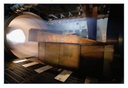
Wind tunnel testing of the X-I demonstrator engine
