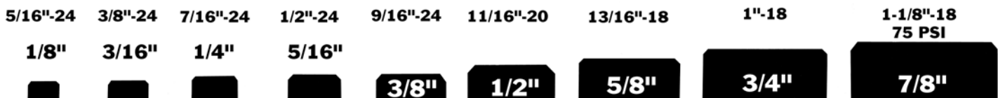
Actual Profile of Compression Threads
