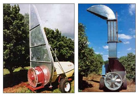
Plate 6. Air-blast sprayers with tower.
