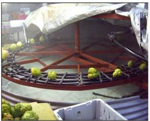
Plate 11. Left: A high pressure sprayers used to clean fruit. Right: A semi-automated system with the fruit sprayed with pressurised water.
