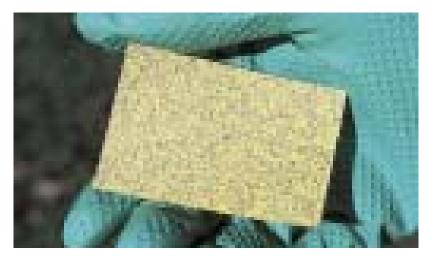
Plate 1. Water sensitive paper that show droplet distribution.
