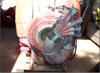
Plate 4. Different types of low-profile air-blast sprayers used by small growers.
