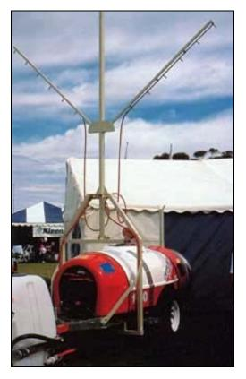
Plate 5. Structurally modified low-profile air-blast sprayers.
