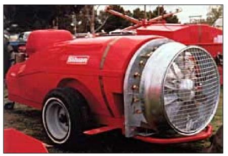
Plate 3. Low-profile air-blast sprayer.
