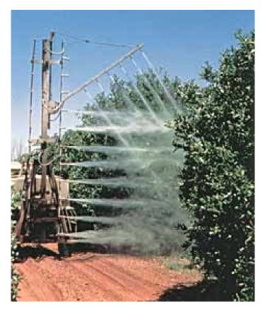
Plate 2. Oscillating boom sprayer.
