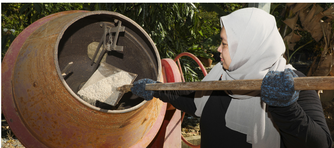
Figure 3.7: Layers of soil and sand are put into the concrete mixer evenly before being sent to storage
