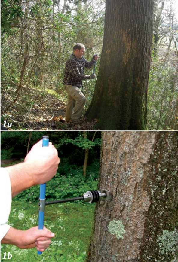
Photos 1(a-b) Sampling from living trees with an increment borer and attached extractor device.
