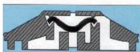
Figure 7. Diagram showing how the membrane works in a self-compensating dripper (Irritol System Europe s.r.l).
