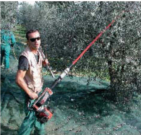
Figure 17. Mechanical hand-carried shaker.
