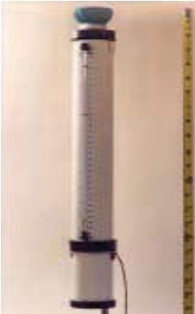
Figure 2. Atmometer (from Altenhofen, 1985)
