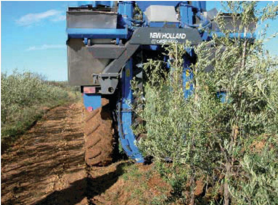
Figure 31. Superintensive orchard with over-the-row harvester.
