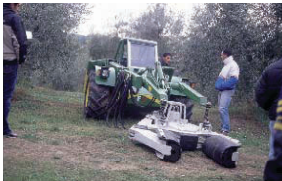
Figure 22. Shaker with two eccentric masses and one hydraulic engine.
