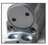
Latching and Sweep Adjustment Valves
