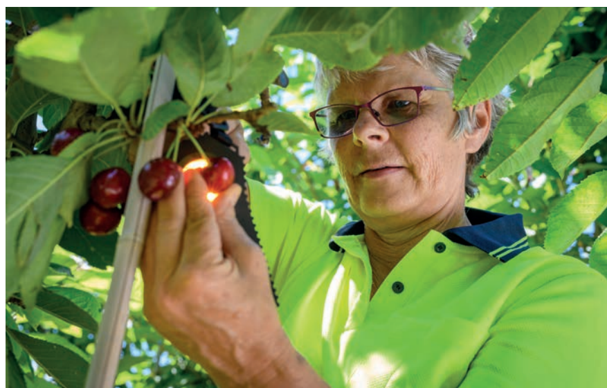
› Jill Stanley measuring cherry fruit quality in the field using a Felix F-750 spectrometer at the Clyde Research Centre, Plant & Food Research. Photo by Craig Robertson, Plant & Food Research.
