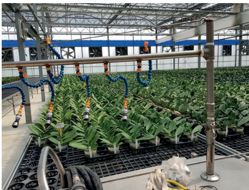
■ Figure 5. Ground self-propelled automatic watering machine in a greenhouse of I-Hsin Biotechnology, Taiwan.
