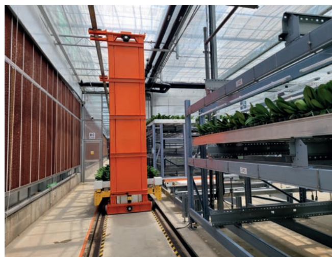
■ Figure 4. Automated storage and retrieval system in a greenhouse at Symon Agricultural Biotech, Taiwan.
