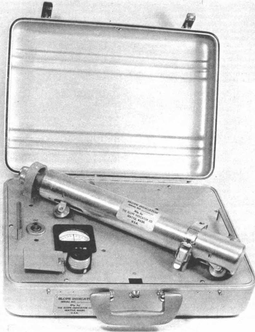
Fig. 50 Inclinometer for Detecting Horizontal Ground Movements
