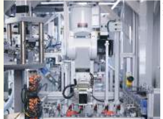
Apple's "Daisy" disassembles and recycles around 1.2 million iPhones a year.
