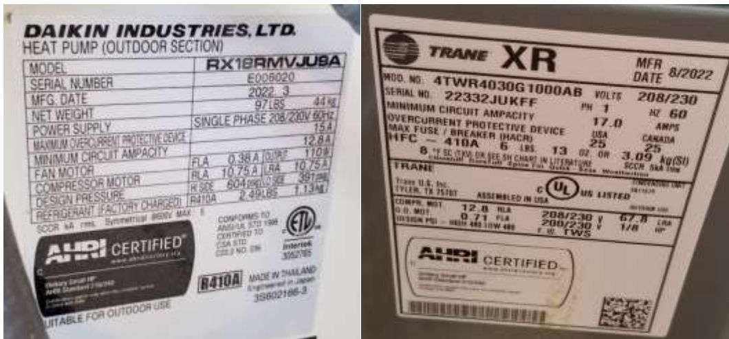
Figure 4: Examples of HVAC Name Plates
