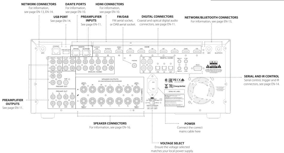
Before connecting your Receiver to your source components and speakers, please read through the next few pages which will explain all the input and output connectivity that is available. The 'Speakers' section explains how to connect up your speakers to avoid damage to the amplifier and how to arrange your speakers for best performance.
