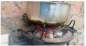
Figure 5. Briquette testing in KCJ cookstove
