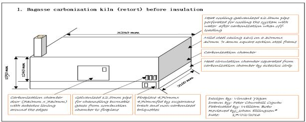
Figure 3. Sketch of bagasse biomass carbonization kiln
