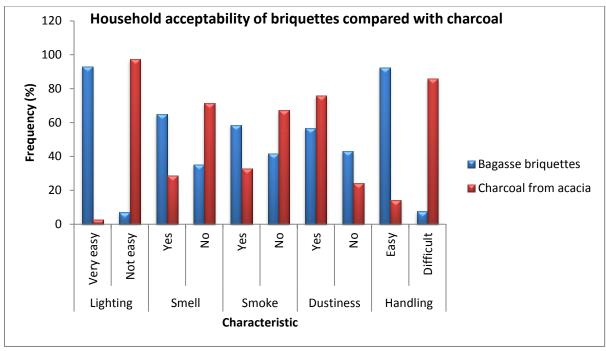
Figure 12. Characteristics of briquettes and charcoal for household use
