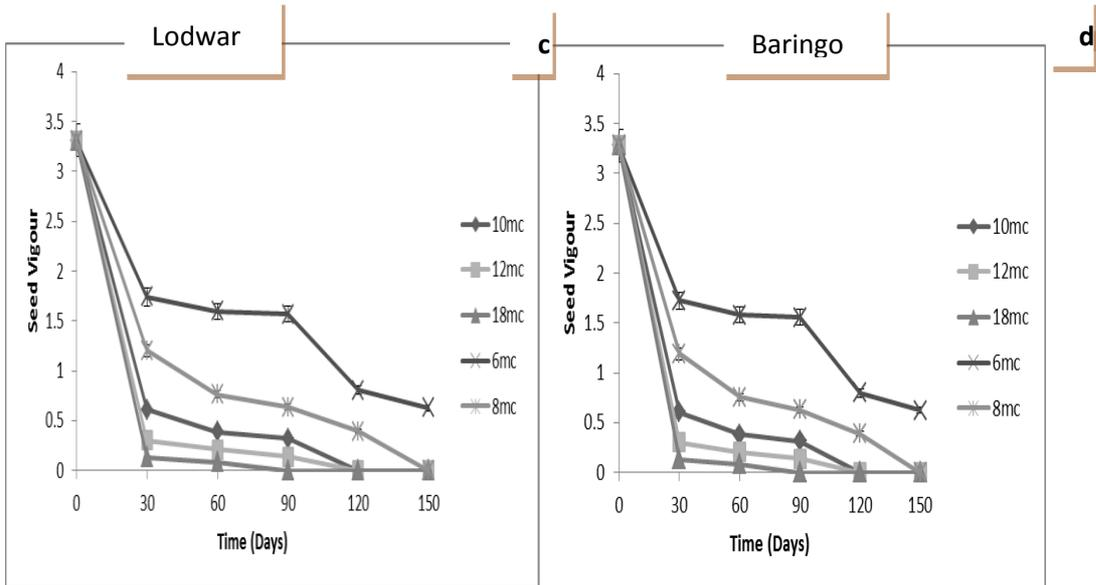
**Figure 4b.** Seed vigour and longevity stored at 35 °C for 150 days
