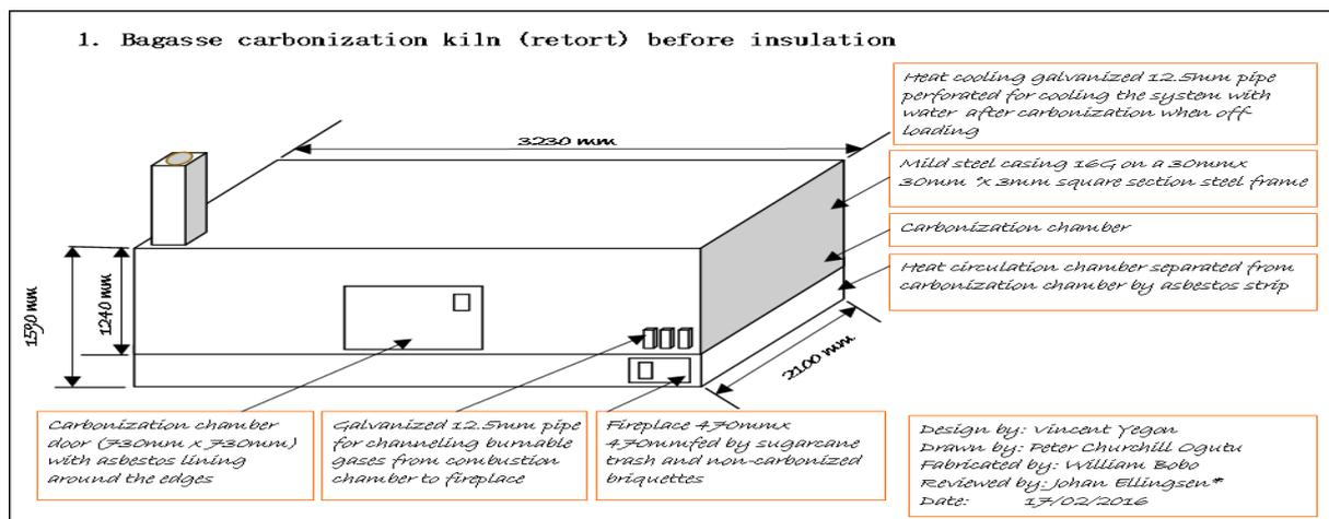
**Figure 3.** Sketch of bagasse biomass carbonization kiln
