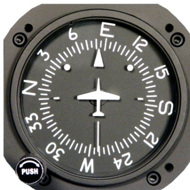
RCA11A-15 P/N J8000-11 Features Cardinal Heading markers N., S., E. & W. (Piper/Cessna display)
