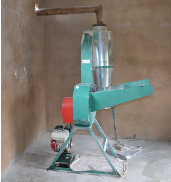
Figure 3 – Hammer mill machine used for processing the plant. (Photo: S. Ngwako, BUAN.)
