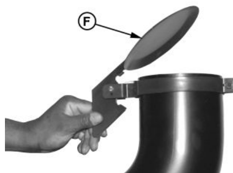
Exhaust Stack Rain Cap
