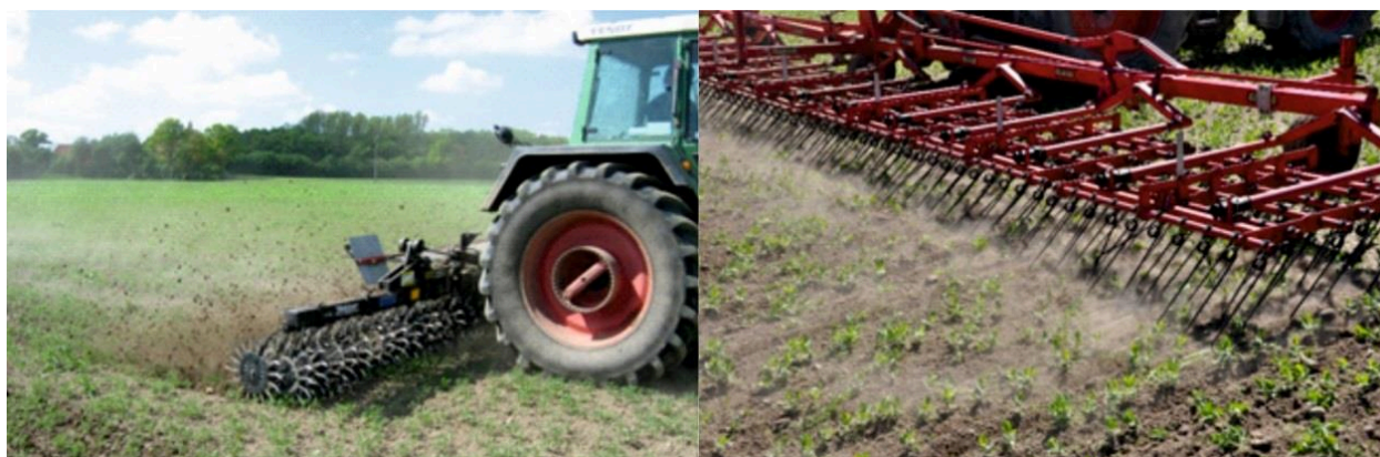
Figure 6. Possibilities of mechanical weed control in legumes. On the left: Use of a rolling harrow in Blue Lupines; right: Use of a chopping harrow in forage peas.
