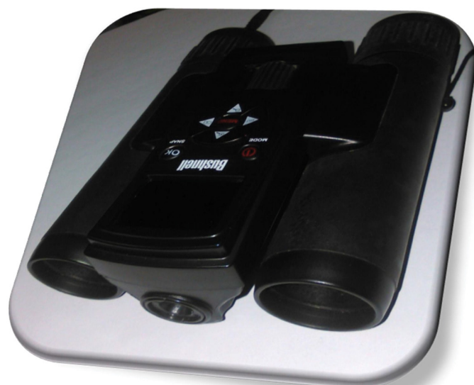
Figure 2: Binoculars with integrated digital camera (Brand: BUSHNELL). (Photo: Sodjinou K. Edjèdu)
