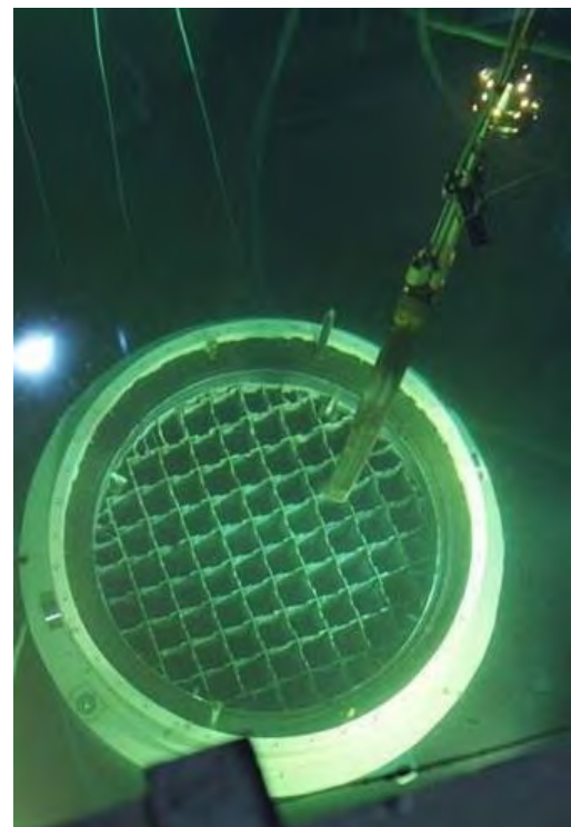
Loading spent fuel cask under water. (Courtesy: Holtec International)
