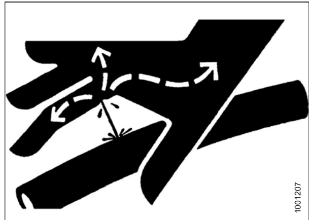
Figure 1.12: Hydraulic Pressure Hazard
