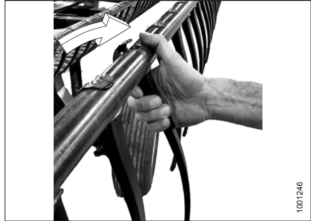
Figure 5.229: Installing Plastic Finger
