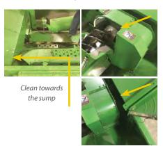
rotor/cylinder, can be key points where plant material can accumulate. Blowing out plant material can be a bit timeconsuming but is well worth the effort in order to reduce the risk of contamination of soybeans in your peas (Figure 4).
