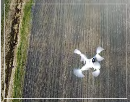
A DJI Phantom 4 Pro equipped with a multi-spectral sensor conducts an early-emergence diagnostics flight on a field near Winnipeg, Manitoba in May, 2020.
