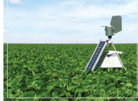
Figure 2. A cyclone sampler collecting air samples in a bean field in southern Alberta.
