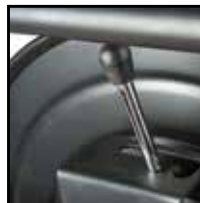
3-Position Brake Lock
