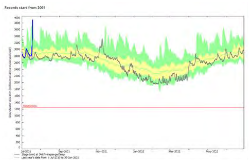
Figure 9: Confined coastal Wairau Aquifer opposite Rarangi representing pressurised groundwater at 40 metres depth. Groundwater levels rose by just over one metre due to a combination of pressure effect from river recharge but mostly loading of Wairau River channel squeezing aquifer with low barometric pressure. Highest level observed since site established in 2000. Some damage to well water level recorder instrumentation caused by natural rapid rise in well levels, explaining why record stops abruptly. Similar response at MDC Bar Well 1733 north of Wairau River mouth.
