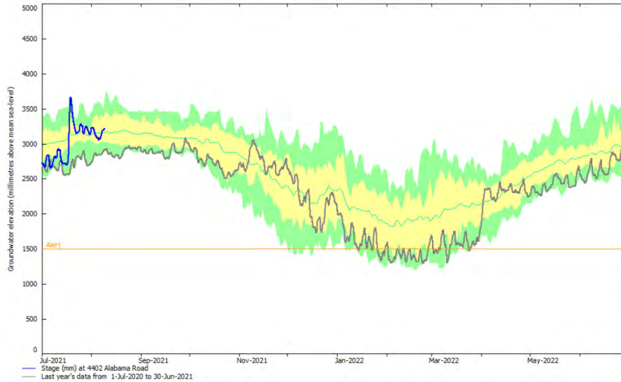
Figure 11: Inland confined Riverlands Aquifer at MDC Well 4402 off eastern end of Alabama Road. Similar response to Lagoon well representing Riverlands Aquifer, with a loading effect rather than effective recharge.
