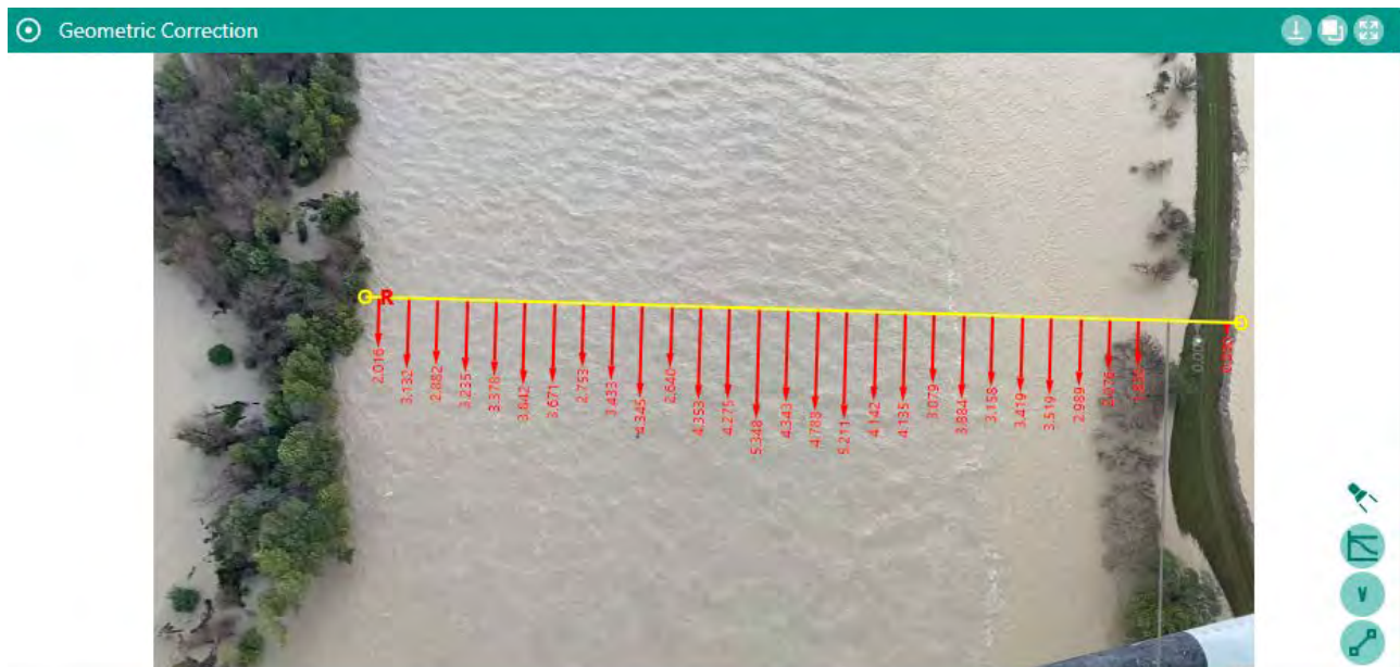
Figure 2: Wairau River at Barnett's Bank (State Highway One) 17 July 2021 at 1750. Screen shot of video taken from a Helicopter over the river that has been analysed using the HydroSTIV software. The red lines are river velocity vectors computed by the software.
