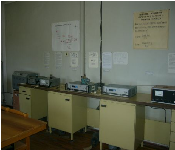
Figure – Gas analyzers to detect and determine the content of carbon monoxide and hydrocarbons
