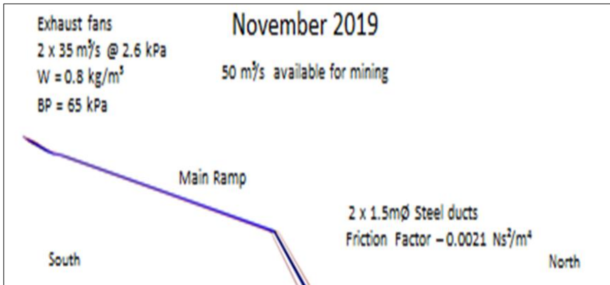
Figure 16-18: Fan Pressure Requirements Main Ramp
