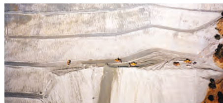
Fig. 12: Construction of terraces (left) and soil covering (right) in the Amiantos Mine area
