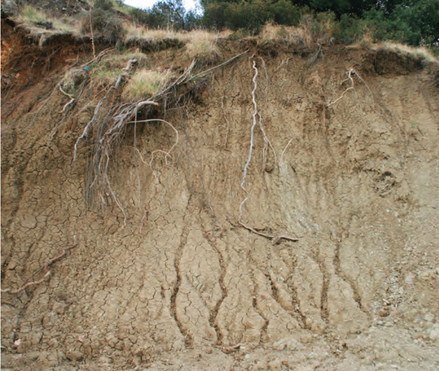
Fig. 54: Intensely disturbed bentonitic clays due to the property of montmorillonite to expand and contract when it absorbs and loses water respectively
