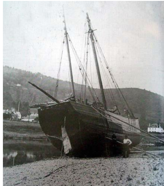
Fig.5 An example of a Trow - a type of flat bottomed boat built in or near the village for use on the river
