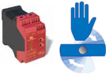
SM125SMS45 detects back EMF of motor and senses when hazardous motion has ceased, then signals guard locking switch to unlock
