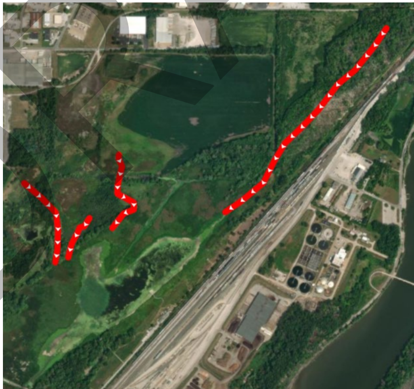
Figure J-3. Flow paths to the Marsh as determined by visual inspection of Green LiDAR data
