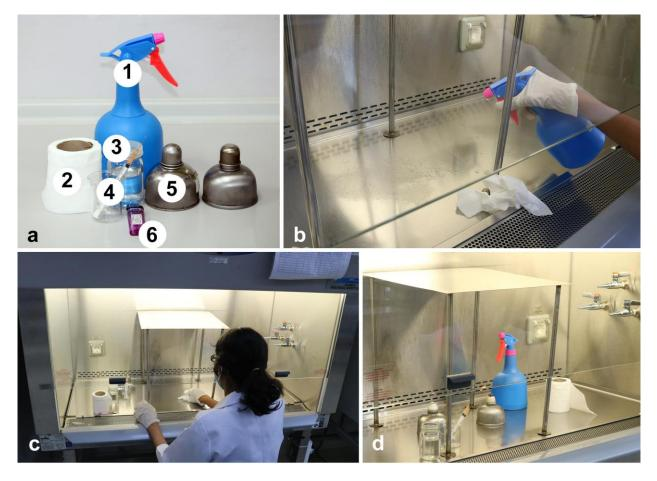
**Figure 3** – Aseptic working bench. a (1) 70% alcohol sprays, (2) Tissues, (3) 70% alcohol bottle for dipping, (4) Needles, (5) Alcohol lamps. (6) Lighters. b, c Surface sterilization of working bench with 70% alcohol. d Common set-up of materials inside the laminar flow.
