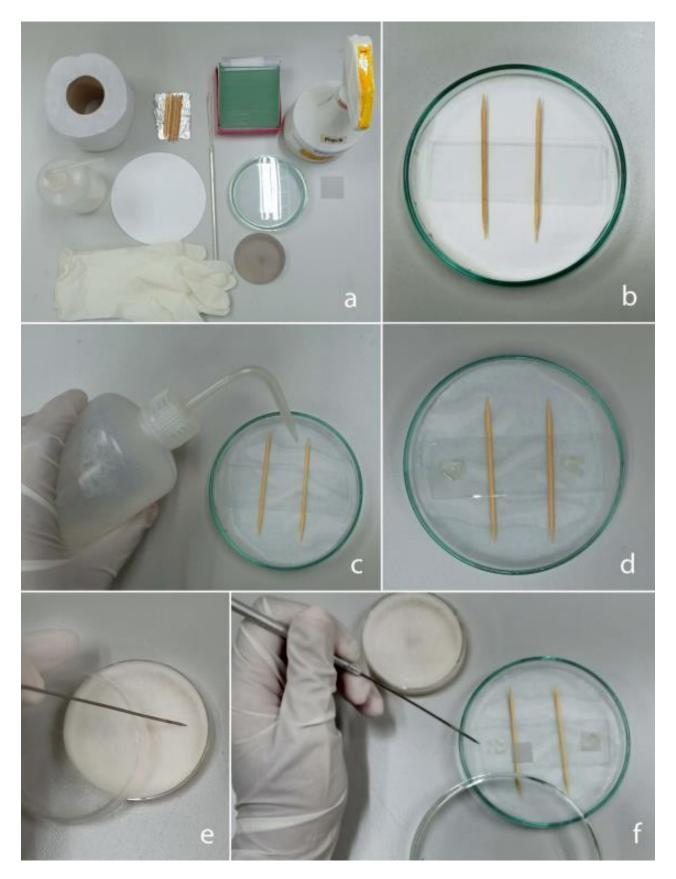
**Figure 7** – Apparatus for slide culture method. a Tools. b Sterilized filter paper, sticks and slides. c Adding sterilized water on filter paper to maintain humidity. d Potato Dextrose Agar (PDA) blocks on both sides of the slide. e Picking a small amount of mycelia. f Inoculation of PDA blocks.
