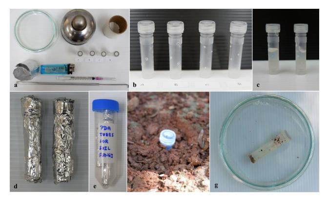
**Figure 29** – Immersion tube method. a Tools. b Screw cap micro tubes with tiny holes. c Screw cap micro tubes with PDA medium. d Aluminum foil-wrapped tubes. e Sterile tubes. f Tubes immersed inside the soil. g Tube transferred to sterile Petri-dish.
