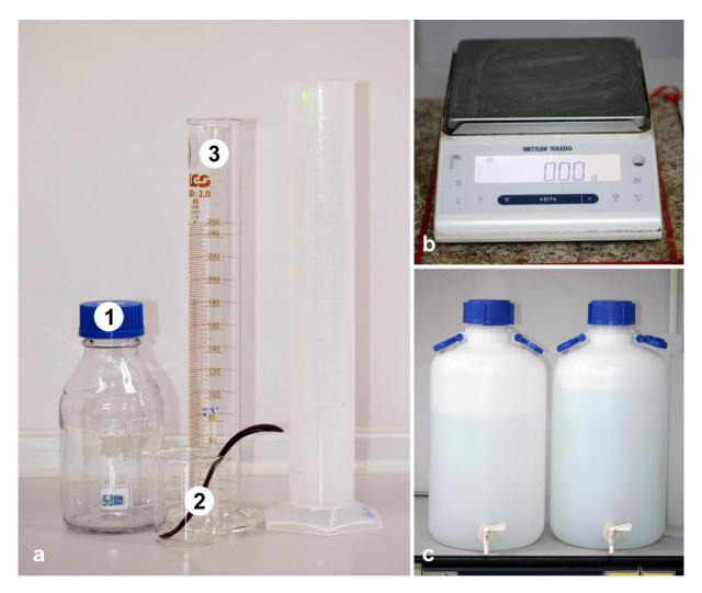
**Figure 14** – Materials and tools needed for media preparation. a Materials used to prepare media (1) Media bottle, (2) Spatula in a beaker, (3) Graduated cylinder. b Precision balance. c Distilled water in polyethylene containers.
