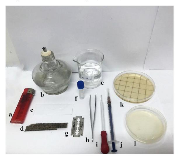
**Figure 17** – Material and tools used in single conidium isolation. a Lighter. b Alcohol lamp. c Microscope slide. d Plant materials. e 70% ethanol. f Sterilized distilled water. g Razor blade. h Forceps. i Pasteur pipette. j Needle with syringe. k 90 mm Petri-dish with marked squares. l 60 mm Petri-dish.
