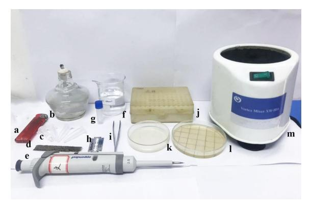
**Figure 18** – Material and tools used in the spore suspension method. a Lighter. b Alcohol lamp. c Centrifuge tube. d Plant material. e Micropipette. f 70% ethanol. g Sterilized distilled water.
