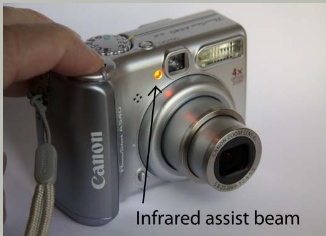
Infrared focus assist beam of P&S camera when the shutter button is depressed half-way.
