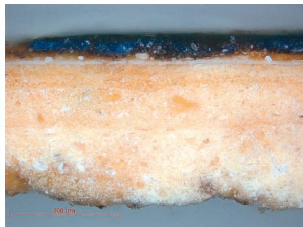
FIG. 15 Paint cross-section of the Virgin's mantle from Leonardo da Vinci, The Madonna of the Carnation (FIG. 35) showing two layers of gesso ( gesso grosso and gesso sottile ) followed by an imprimatura containing lead white. Over this is a translucent brown layer, rich in medium, followed by a thin blackish layer and finally a layer of ultramarine and lead white.
