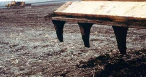
A bulldozer, modified with 'tiger-teeth' attached to the blade, is an effective means of surface modification that promotes root growth by reducing soil compaction
