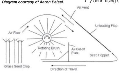
Figure 24: Schematic of a Woodward Flail-Vac © seed stripper
