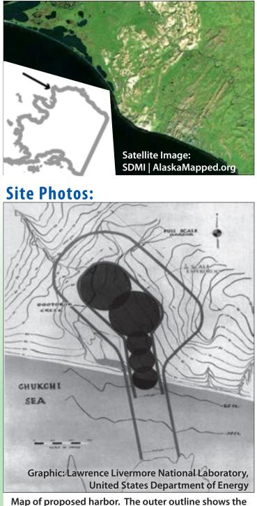
Map of proposed harbor. The outer outline shows the "full scale" plan, with detonations totaling 2.4 megatons. The inner outline, a scaled down version, would have required blasts of 460 kilotons.
