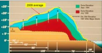
The height of the foredune, when measured in 2009, nearly matched the height predicted in 1998. Also, the prediction of road inundation did come to pass and clearing the road of sand is now a constant maintenance issue.
